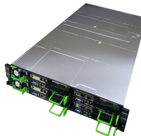
Chassis with 8 nodes, 2U size (Fujitsu PRIMERGY CX600 M1)
